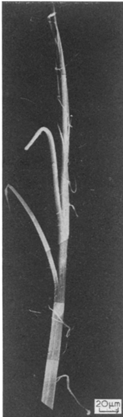
Figure 4 Tensile fracture morphology of Kevlar-49 showing severe splitting.
